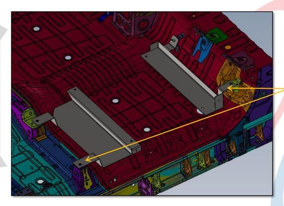
PLACE LOWER SHELF SKIN ON MOUNTING BRACKETS, ALIGN WITH HOLES ON BRACKETS, PLACE LIP FLUSH WITH OUTSIDE OF BRACKET REMOVE REAR SEAT, LIFT FRONT SEAT FROM REAR MOUNTING POINTS.
